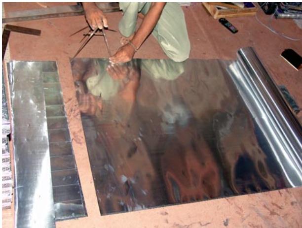
unwrapping aluminum coils and marking sizes
