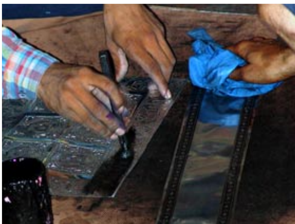
coloring or oxidizing using oil paints and applying brush on the embossed aluminum panels. cleaning surface to remove undesired color.
