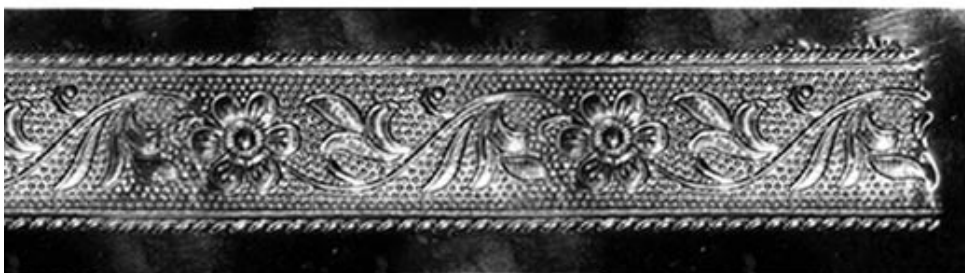
continuous borders made using stamping single die and multiple operation
