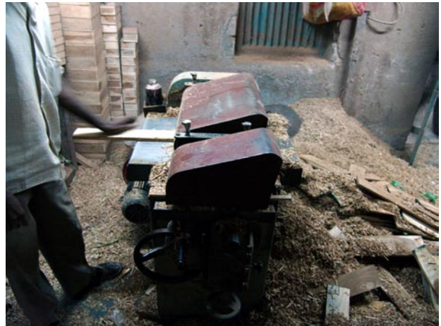
randha machine for smoothening surface
