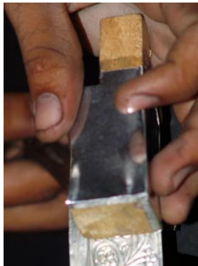
a step by step process showing strapping aluminum metal surface done with mina work for making bajot base
