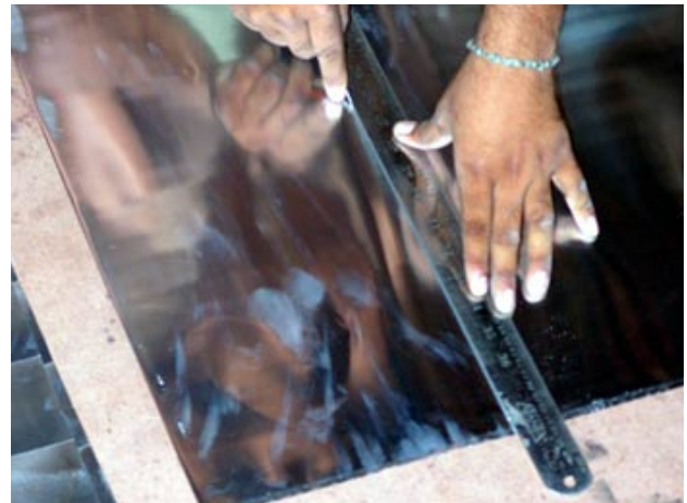
cutting and sizing of aluminum panels as required
