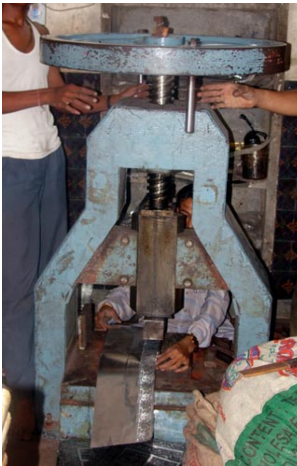
stamping press during the operation of metal embossing. adjusting placements and amount of impact required
