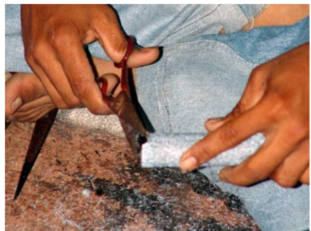
clock wise from top left ; cylendrical wooden bars wrapped with velvet, cutting extra legths, pasting velvet with wooden bars
